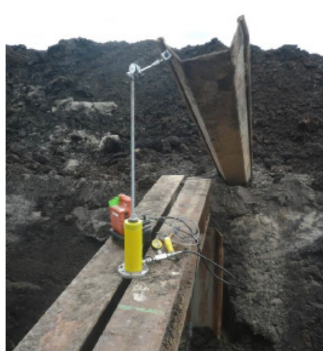
SUBFRAME FOR LONG TERM TEST (according JLD protocol)
