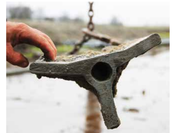
The LDE (fin) element transfers the shear force to the soil.
